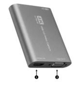
1.HDMI in: Connect to TV or monitor HDMI port 2.VGA out: Connect to VGA monitor VGA port
